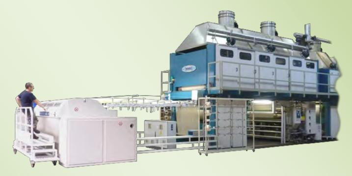
True innovation in comparison to any other traditional sizing system. Simpler concept and easier control compared to conventional yarn dipping with/without a pre-wetting system. It gives better weaving performance and preserves yarn elasticity, whilst being eco-friendly saving a lot of consumables and waste in terms of water, chemicals, drying energy and water/air contamination.
